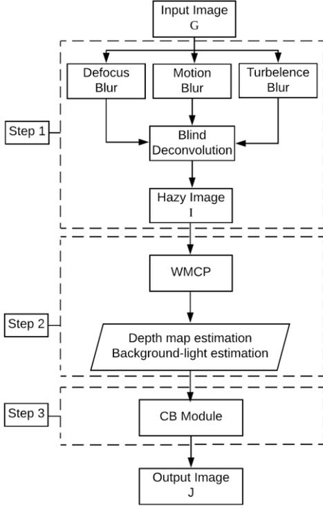
Figure 1. A three-stage flowchart of the proposed method.
